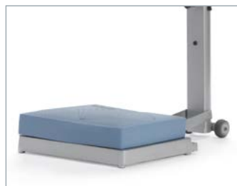
CTSIB Indexed Pad for the Balance System SD (left) and BioSway (right) provide consistent surface for unstable test conditions.
